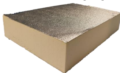
Fig. 2 Flame-retardant polyisocyanurate rigid foam demonstrator containing T(nBu) 3
