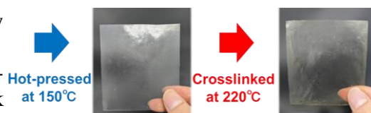
Fig. 5 The hot-pressed film and the crosslinked film of \alpha -1,3-glucan-BH
