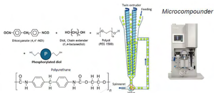
Fig. 1 Reactive extrusion of thermoplastic polyurethane using a microcompounder, adapted from [3]
